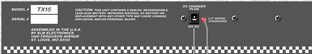
**13. DC CHARGER PLUG:** Use this jack to connect the 15VDC charger to the amplifier to recharge the battery (power switch off) or to supply power to the amplifier while playing (power switch on). Plug the charger into an AC outlet of the proper voltage as listed on the charger.
