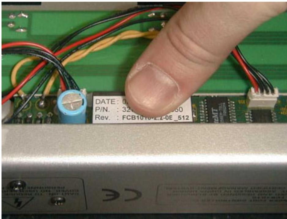
Fig. 3.3: Placing the new EPROM
