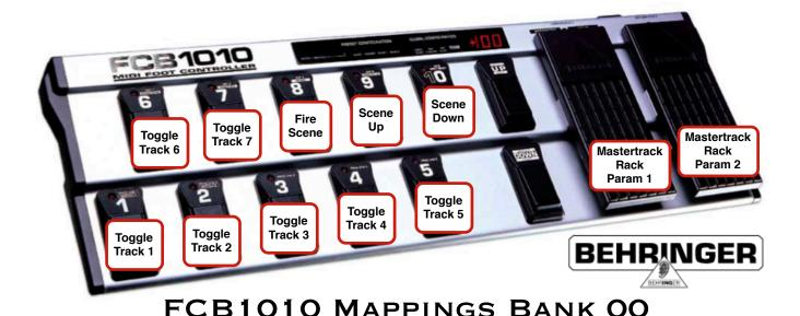
The banks "01" through to "09" are assigned to a track. Bank "01" controls the first track in the current set, bank "02" the second, and so on up to the ninth track. This also works when tracks are added, deleted or moved. The mappings for the track banks are as shown in the graphic below:
