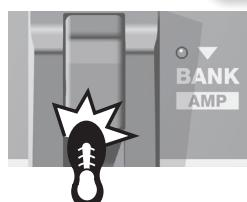
When In Manual Mode and Memory Edit Mode, use the [BANK ▼]/[AMP] pedal to turn on and off.
