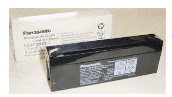
We tested a Panasonic LC-R122R2PG battery, 12 V 2.2 Ah, which can operate the QuadMic for 4 hours. Measuring the voltage while discharging shows that the QuadMic remains completely in working order even shortly before the battery voltage collapses (6 Volts.)
